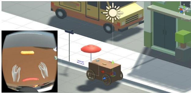
Fig. 2. Orthographic view of the virtual scene as seen in the development environment. A picture-in-picture view shows the virtual environment from the user's perspective (with a bun and hotdog as the reaching goal and interactable object respectively). The axes origin shown behind the hotdog cart matches the axes in the physical space marked in Fig. 1.
